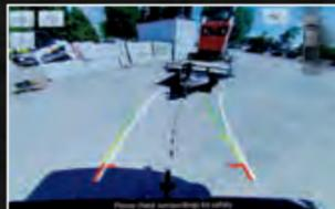
**REAR VIEW CAMERA WITH DYNAMIC HITCH ASSIST**
