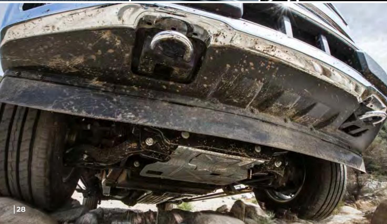
"FX4 Off Road" decals on your pickup box let everyone know you're capable of serious, off-road travels. On XL through PLATINUM 4x4 models, the FX4 Off-Road Package equips your truck to get out there with an electronic-locking rear differential, underbody skid plates that help protect the front differential, transfer case and fuel tank, Hill Descent Control, and off-road-tuned shock absorbers. Monitor the action from the driver's seat on the off-road display in the productivity screen.
