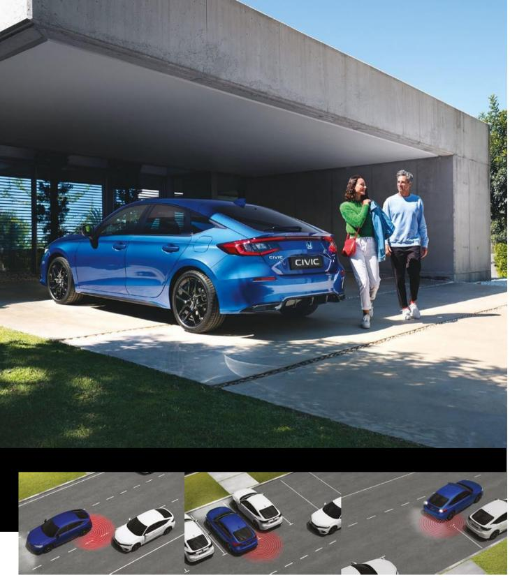
**Blind Spot Information** Making lane changing safer, a discrete warning light is activated in the appropriate door mirror when a vehicle is detected approaching in an adjacent traffic lane.
