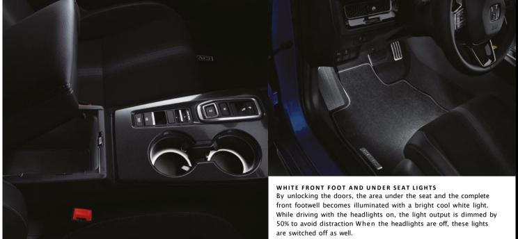
WHITE CUP HOLDER AND CONSOLE ILLUMINATION By turning on the ignition and headlights, the bottom of the cup holders and the storage box in the centre console become illuminated, bringing a cool white light to the interior of your car.
